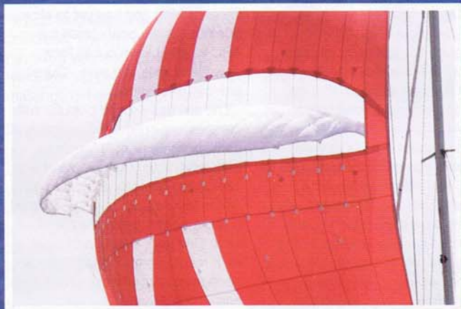
A complex web of lines supports the wing at the correct angle, yet the loads induce no distortion in the sail
